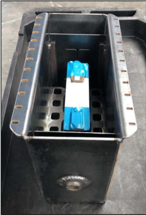
Figure 9: Liquid Immersion Test setup with Battery in AmpCool™ AC-100
